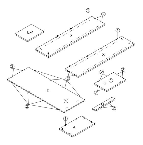
Preparation for Top panel A,bottom panel G,Left side panel X,Right side panel Z,back panels D,Batten O.
